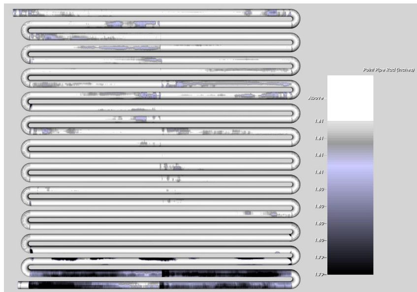
Figure 2: Pass 4 Radiant Coke Scan.
